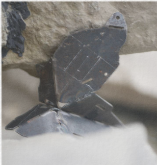
▲ Piece B is developed in an identical way to Piece A, simply utilising a different part of the Steel jig (Section 1.3)
