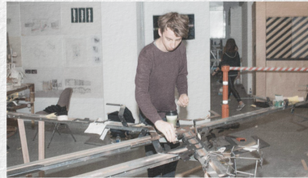
◀ Unit 8 Show (2016) 12mm Aluminium extrusion fixed to 15mm birch ply beams.
